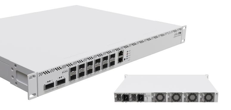
There are **2x QSFP28** cages for blazing-fast 100 Gigabit connectivity, **12x SFP28** cages for 25 Gigabit networking, and a **Gigabit Ethernet** port. The device comes with **16 GB of RAM**, decent **NAND** storage, and **two M.2 SATA slots** for additional storage. There are four hot-swappable fans, as well as dual-redundant hot-swap power supplies. And these PSUs might look familiar if you have used our CCR1072 before: you can keep using your previous hot-swap power supplies and SFP modules.
