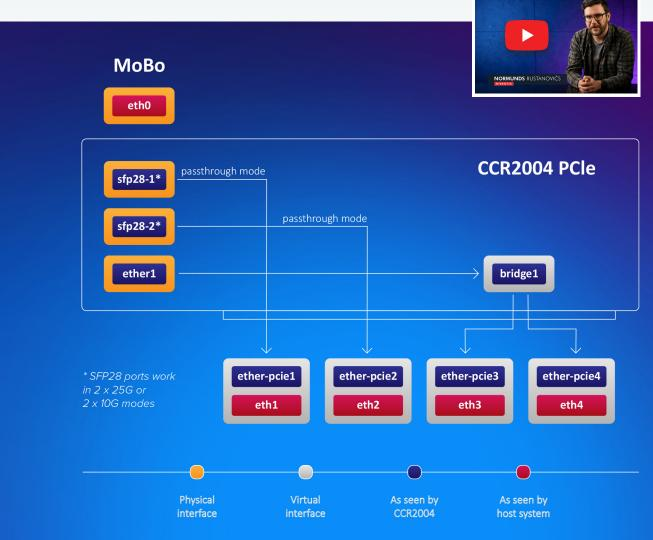
To get this CCR device to work as an NIC, a new Passthrough mode was implemented. Basically, a FastForward FastPath mode that can also pass hardware link statuses.
