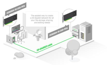
This form-factor does come with certain limitations that you should keep in mind. The CCR NIC card needs some time to boot up compared to ASIC-based setups. If the host system is up before the CCR card, it will not appear among the available devices. You should add a PCIe device initialization delay after power-up in the BIOS. Or you will need to re-initialize the PCIe devices from the HOST system.
